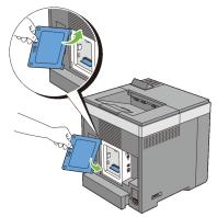
6 Close the control board cover and turn the screw clockwise.
